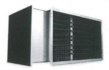
Duct heaters are designed to heat clean air in ventilation systems and to preheat air handling units. Corrosion resistant casing with excellent thermal reflectivity is made from AluZinc. Duct connection is with rolled rubber seals, duct heater elements are made from stainless steel. To ensure safety in duct heaters are installed 2 protection thermostats and screw terminals for easy connection.
